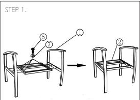
ssemble the seat frame (2) to the steel arm frames (1) with seat screws (5) & washers(7) but do not fully tiahten
