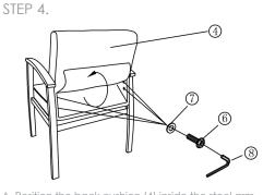
A. Position the back cushion (4) inside the steel arm frames (1) as shown making sure the upholstery is facing forward. Lift up the upholstery at the bottom of the back to expose the back screw fixing points as shown in the drawing. Assemble the back cushion to the steel arm frames using back screws (6) and washers (7) and firmly B. Fully tighten all the seat screws (5) to
