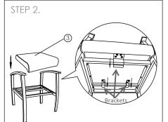
Carefully position the seat cushion (3) onto the seat frame (2) making sure the waterfall front edge of the seat is facing forward matching the drawing as shown.
